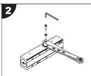
Arm is fitted in pinion with hex head screws.
