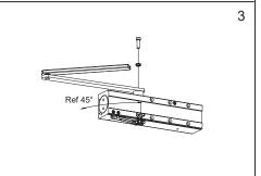
Rotate the bottom pinion to approximately  $45^{\circ}\,$ with a wrench as illustrated and then assemble the main arm.
