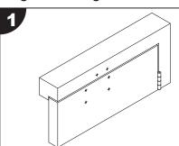
Using the templates provided, mark and drill pilot holes into the door and frame.
