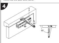
Attach the armset to the mechanism ensuring the pre-loading requirement has been completed.
